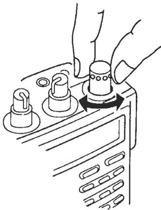
To change the frequency in 100 kHz steps, hold down the FUNCTION button while you turn the ROTARY CHANNEL SELECTOR.
